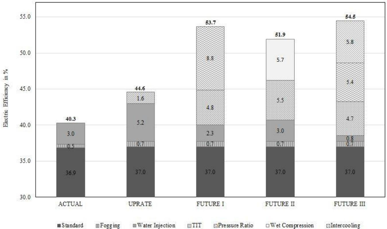
Fig. 5. Potential improvements of HiTES cycle efficiency [6]
