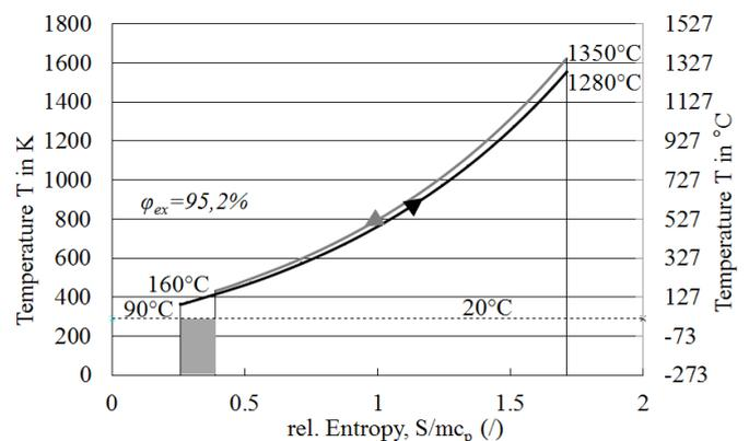
Fig. 2. Entropy increase during the heat transfer in a Pebble-Heater
