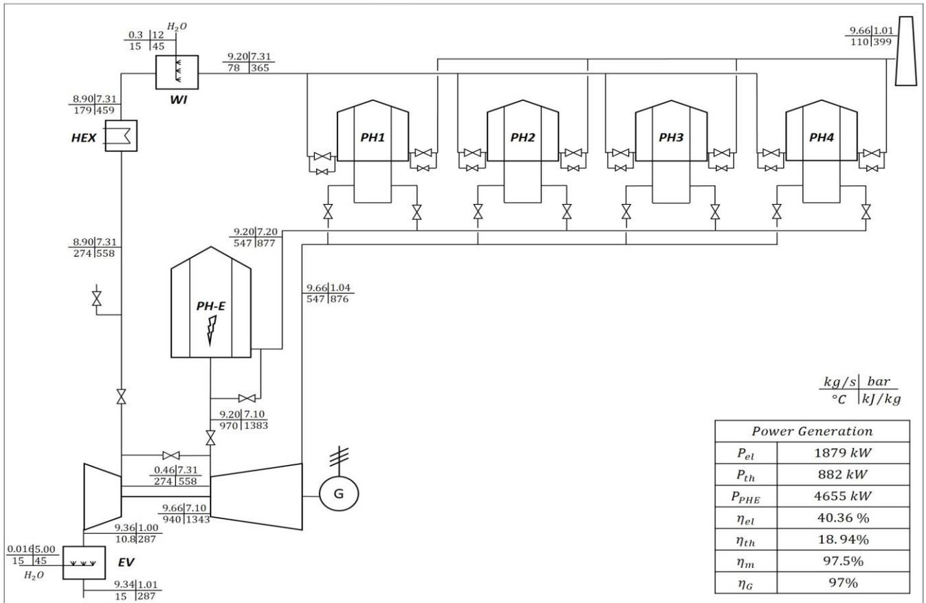
Fig. 4. Flow diagram and nominal process parameters of HiTES
